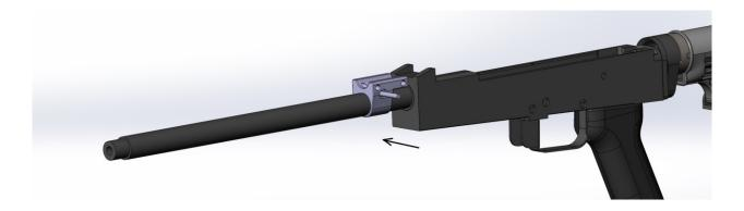
Slide assembled upper (with iron sight base and dustcover insert) on to the barrel nut. Fix it with 2 front screws (a.) and two rear screws (b.) to the Barrel nut. While fixing upper with crews do control that upper should be parallel to the bore or have slight incline forward)
