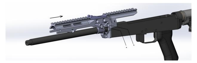
In case of Chinese AK or Vepr (RPK) rifles with wider front trunnion and trickier receiver walls you will need to file down areas on the "tooth" (a.) and "ears" (b.) to fit.
