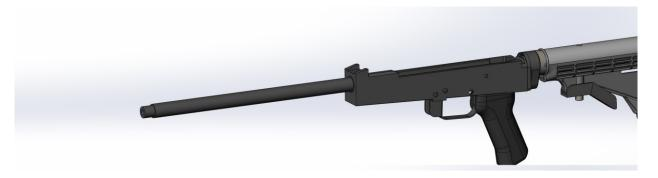
Pressfit the provided barrelnut on to the barrel till the side hole for fixing pin will not align with the cutout on the barrel left after you removed the rear sight post.
