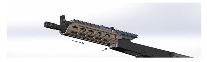
Insert BCG into place and install the recoil spring. Check the charging function.
