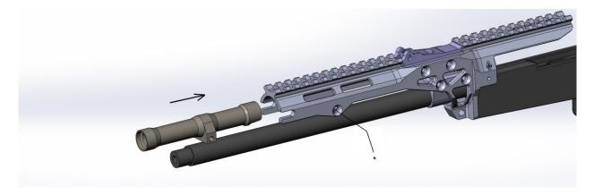
Make sure fixing is not stiff and allows gas tube rotate on the screw axis up and down to compensate barrel harmonics during the shots string.
