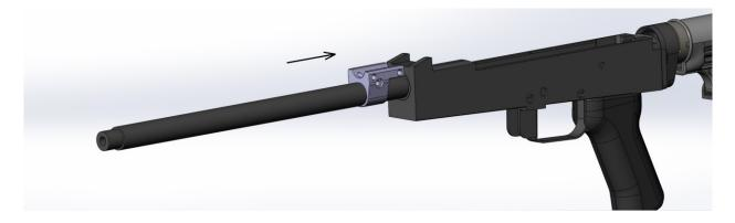
**STEP 4**Pin the barrel nut with the barrel nut pin
